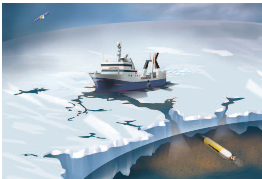
Fig. 2 A combined effort involving multiple sensor-carrying platforms such as AUV under sea ice, remote sensing from a polar-orbiting satellite and a research vessel allows for a more holistic view on productivity in ice-covered waters than previously possible. Each platform is equipped with an array of sensors giving bio-geo-chemical-physical information over larger areas and depths
