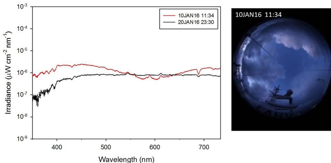
**Figure 17.** Representative spectral irradiance data for skylight dominated by sun and moon. An all-sky image for approximately solar noon on 10JAN16 is shown at right.
