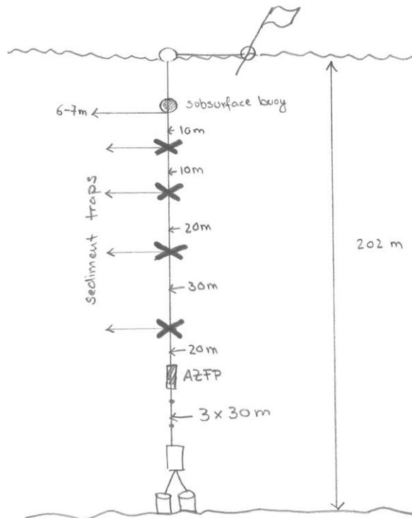
**Figure 10:** Drawing of the setup of the mooring. A depth meter was deployed right under the subsurface buoy, and indicated a depth of 6-7 m (low/ high tide).
